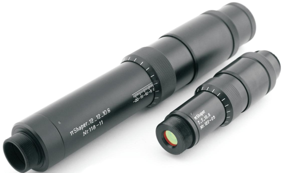
With these unique tools it is possible to convert a single mode or multimode laser beam of similar to Gaussian intensity profile into a collimated Flattop beam with nearly 100% efficiency.
